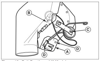
Figure 15. Belt Routing - 44" Models
